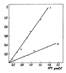
Fig. 2. Standard calibration curves for dyes in tricresol: ( $\Box$ ) dye (a), concentration 1.7  $\times$  10<sup>-5</sup> gmole/l. in red filter; (O) dye (b), concentration 3.4  $\times$  10<sup>-5</sup> gmole/l. in red filter.
