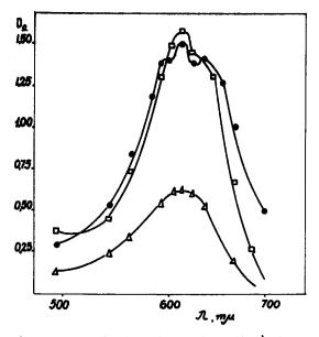
Fig. 1. Absorption spectra for dye (a) and colored PEGT (solution in tricresol):  $(\Box)$  pure dye (a), concentration  $4.10^{-2}$  g/l.; ( $\bullet$ ) pure dye (a), heated, concentration  $4.10^{-2}$  g/l.; ( $\Delta$ ) colored PEGT, concentration  $8.10^{-2}$  g/l.
