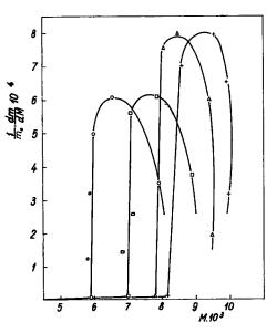
Fig. 3. Differential distribution curves for colored PEGT (from 0.1% tricresol solution): (O) dye (b), concentration in reaction mixture 0.5%; ( $\Box$ ) dye (b), concentration in reaction mixture 0.25%; ( $\Delta$ ) dye (a), concentration in reaction mixture 0.5%; (+) dye (a), concentration in reaction mixture 0.25%.
